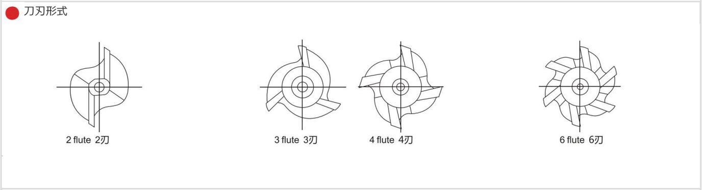
Shape in end teeth of the end mill 立銑刀的底刃形狀
